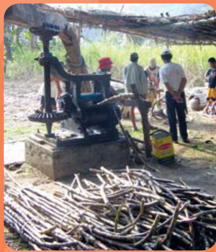
An indigenous community of La Union uses an iron press to squeeze sugar cane juice to be cooked into natural sugar. Traditionally, the dapilan or sugar cane press was made of two upright logs, powered by a carabao. The sticky cooked sugar is poured and set to cool in coconut bowls. The result is solidified bowl-shaped sugar that is consumed by the family. Surplus is sold in the market.
