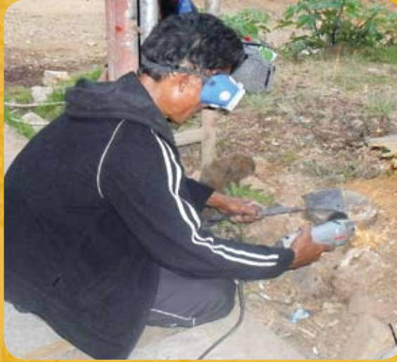
An indigenous blacksmith polishes a small axe with the use of an electric powered grinder. Traditionally, the axe was polished by hand with the use of a file. The axe is a multi-purpose implement used to cut trees and underbrush to prepare the land for planting rice.
